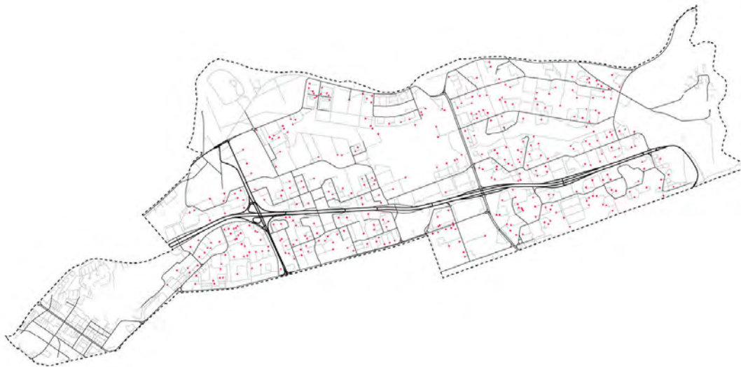
Incomplete network and dead ends: The block size within Lasnamäe is considerably huge compared to blocks in city center or other housing districts in Tallinn. What makes those huge urban blocks even more challenging is the lack of subdivision of neighborhoods. In Lasnamäe, the infrastructure that defines the urban block effectively also defines a neighborhood, which is out of scale. In other parts of the city, smaller subdivisions can be found within the urban block to create a more human-scale neighborhood.
