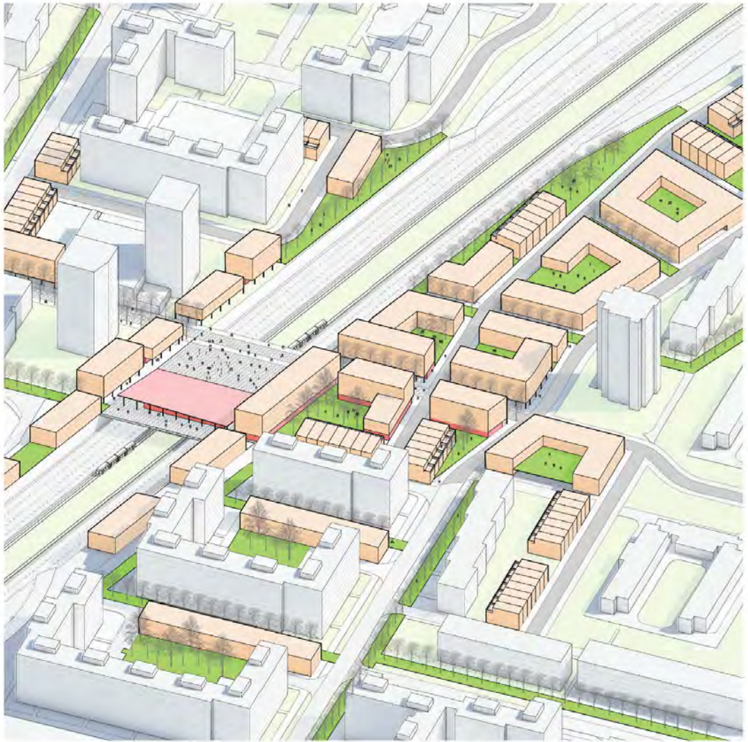
Laagna Axonometric: An axonometric drawing of Laagna center with our proposed interventions realized. Yellow represents new residential development. Red represents new commercial development.
